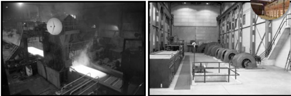
From the people of the steel industry, to the process! This complex of buildings was home of the 120" rolling mill. Like a rolling pin and pizza dough, this machine flattens and thins hot, large pieces of steel. But instead of rolling dough on a kitchen counter, mills roll steel wide and long enough for bridges and skyscrapers.
