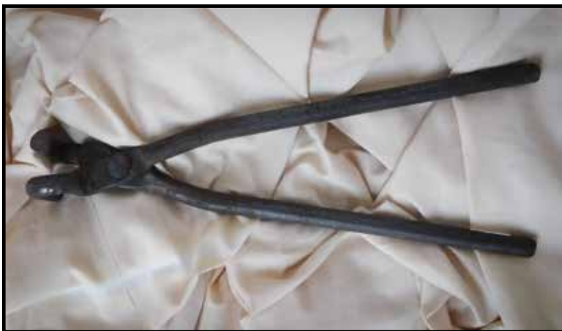
2016.91.1 Hardy tool (fit in Hardy hole) used at Lukenweld blacksmith shop donated by Charlie Rhoads
