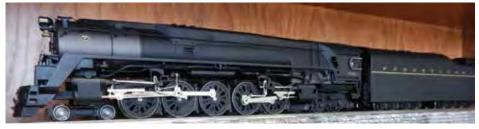
The PRR's class Q1 comprised a single experimental steam locomotive for freight service, #6130, built in March 1942. A duplex locomotive, it had a wheel arrangement of 4-6-4-4, comprising a four-wheel leading truck, two sets of driving wheels (six followed by four) in a rigid locomotive frame, and a four-wheel trailing truck.
